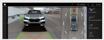
■ Parking Assistant makes parking the vehicle easier. The Reversing Assist camera provides a clearer view behind the vehicle. Parking Assistant parks the vehicle automatically, parallel to the street. The Reversing Assistant supports the driver when reversing. Active Park Distance Control helps prevent or minimise damage while reversing.
