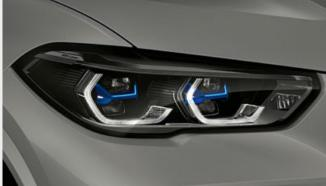
☐ In laser high-beam mode, BMW Laserlights have a maximum illumination range of up to 500m, nearly twice as far as that of conventional headlights. Better visibility in the dark significantly increases safety. The Blue X signature and the 'BMW Laser' lettering underline the vehicle's technological standards. Available as part of Visibility package.
