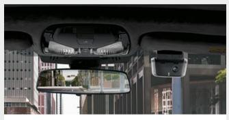
O The **BMW Advanced Car Eve 2.0** is a highly sensitive full-HD camera that captures situations in front of and behind the car, even when it is parked. In the event of disturbances outside the vehicle, the camera automatically records the occurrence in order to document possible
