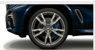
■ 22" light alloy V-spoke style 747 M wheels, Bicolour, front 9.5 J x 22 with 275/35 R22, rear 10.5 J x 22 with 315/30 R22 tyres. (Standard for M50d and M50i models).
