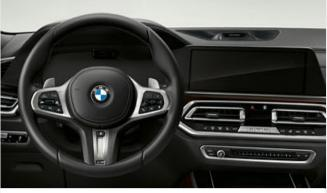
■ BMW Live Cockpit Professional consists of a 12.3" Control Display and a fully digital 12.3" instrument display.
