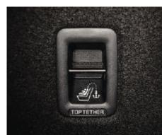
Child Anchor Keep your child safely and securely seated by strapping their seat to the vehicle using straps from the child safety seat that connect to special metal anchors in the vehicle.
