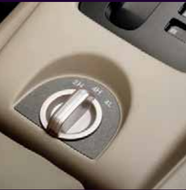
2- to 4-Wheel Drive Switching from 2WD to available 4WD is as easy as turning the knob on the center console.
