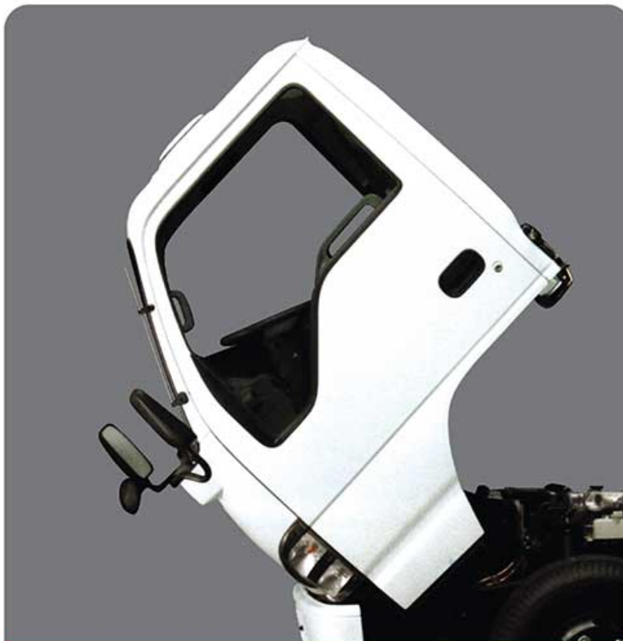
Tilt-cab Design for easy Service (NKR & NPR)
